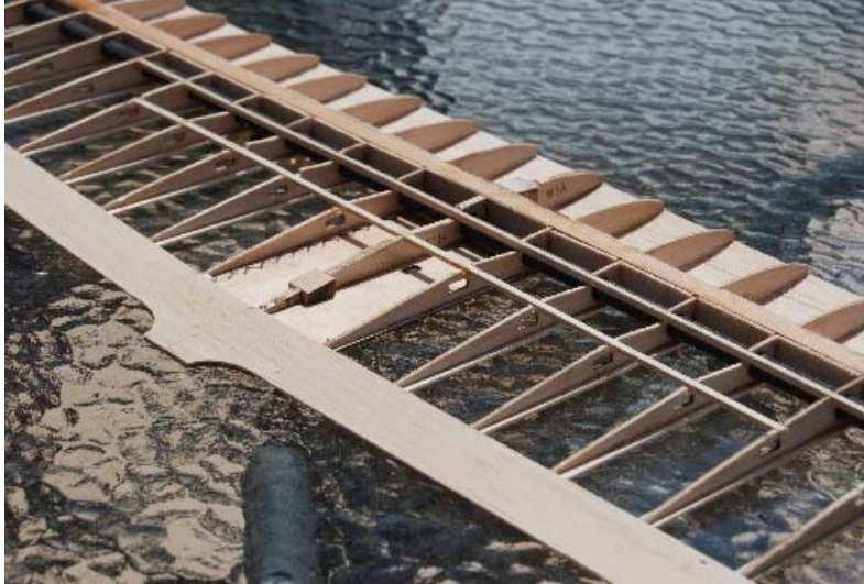
Figure 7. Center Panel Modified for Spoiler
