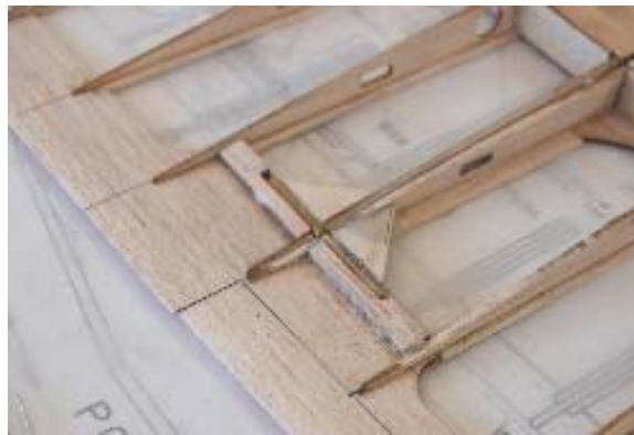
Figure 6. Wing Joiner Alignment Pin
