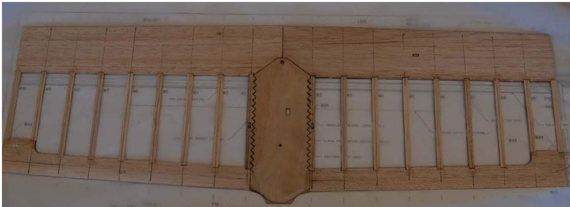
Figure 1. Center Wing Panel Construction
