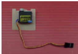
Low tack tape on Servo, servo glued to plate
