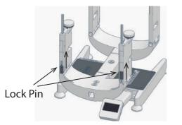
Pin Position: Up to fold; Down to lock.
