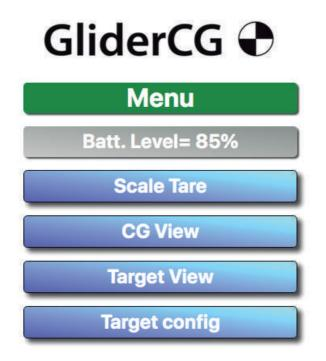
The first menu option "**Scale Tare**" allows you to zero the weight measurement or tare the scale.
